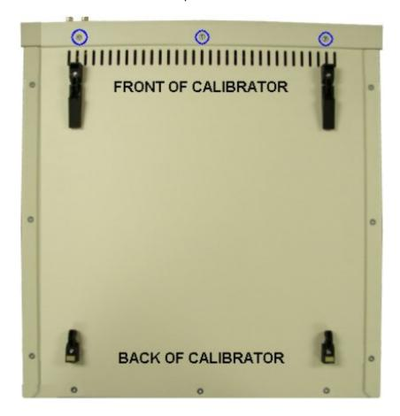
Screws marked in blue hold the bottom of the **front panel** in place. These only need to be removed to allow the front panel to be dropped down. \*\* It is not necessary to remove these screws to remove the top cover from the calibrator case.
